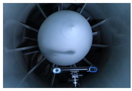
test configurations. It also results in more accurate data with the object under test not needing to be instrumented with contacting sensors. Using advanced tools such as full field strain maps and Rigid Body Motion correction also increases the data capture.
